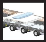
The variable positioned bolsters are controlled through the steering program.
